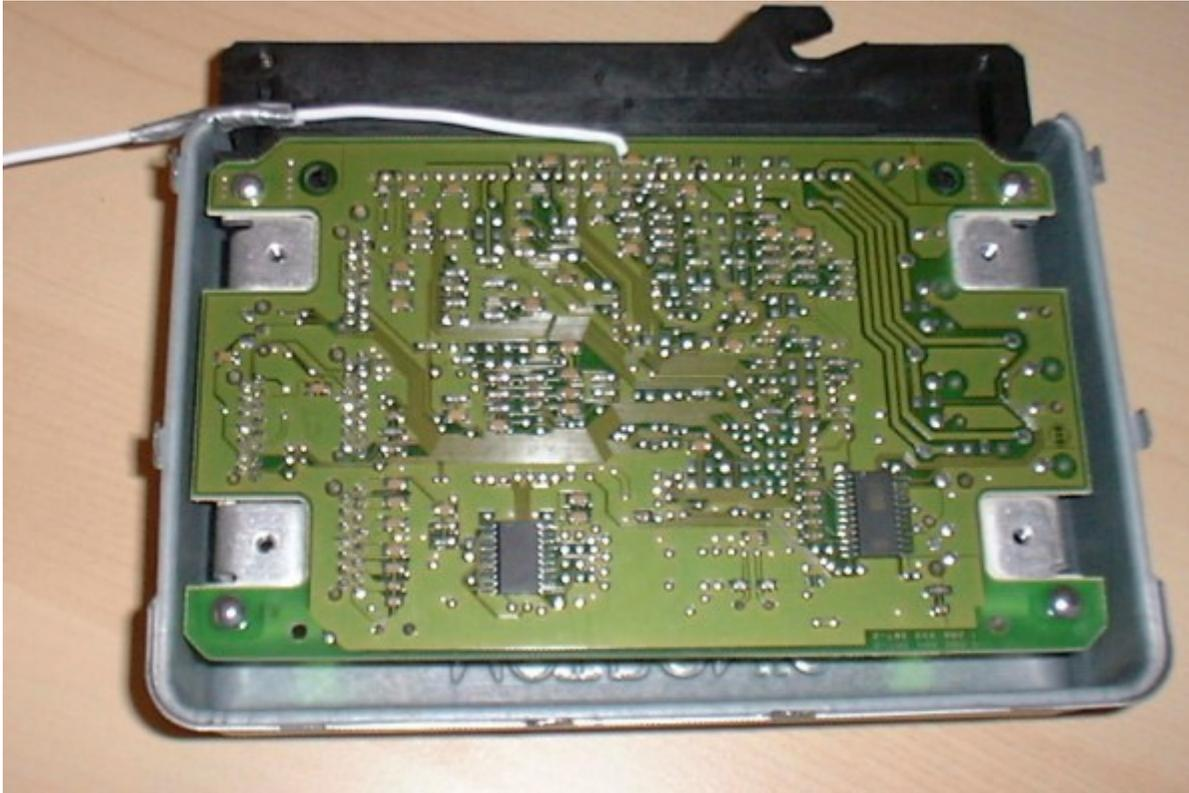
You have to remove the ECU (4 x 10mm bolts) and disconnect the main loom connector, then twist up the metal tags and unscrew the bottom metal panel from the ECU.
