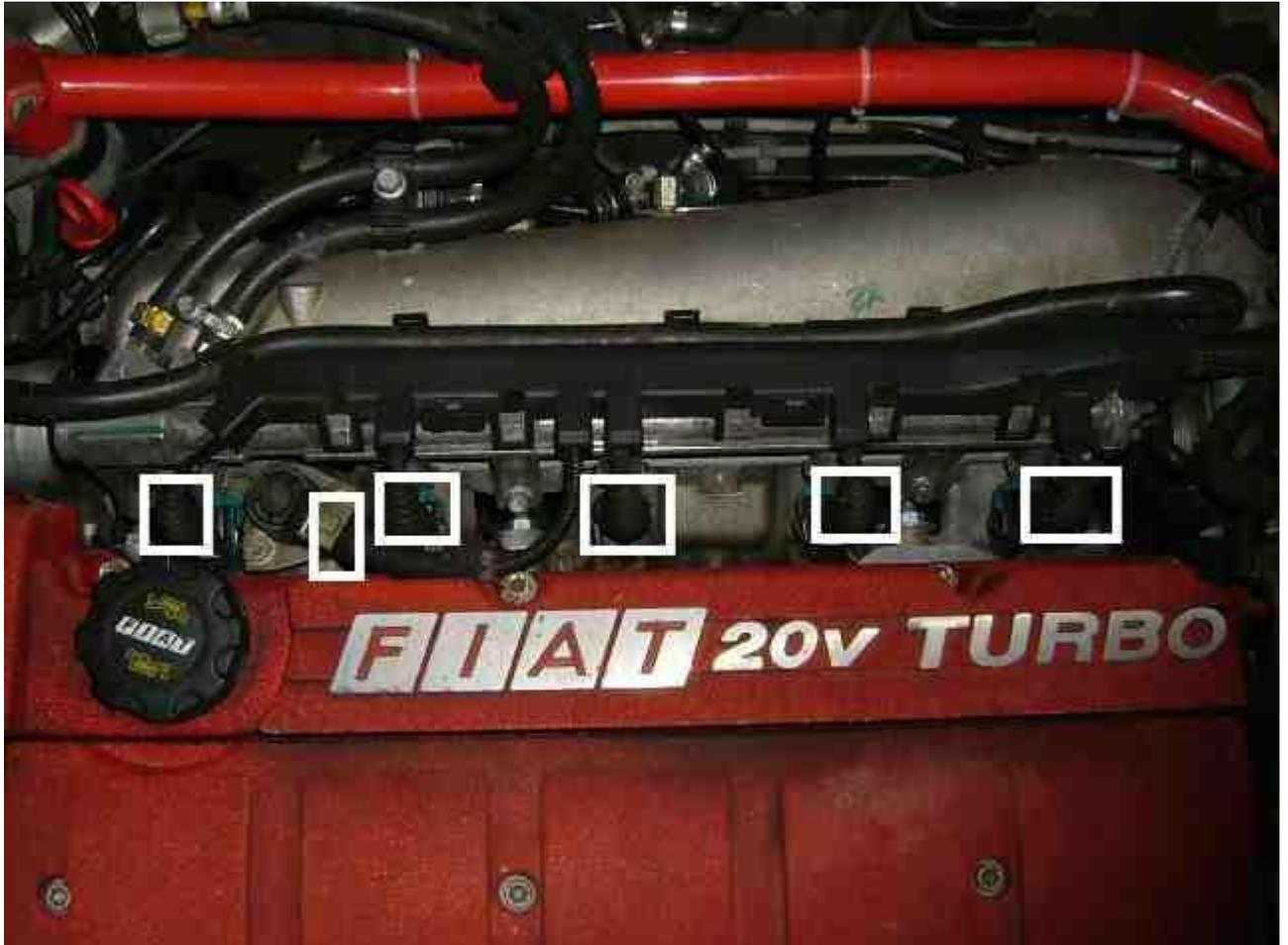
Then undo the hose from the coolant header tank and the fuel hose clip on the back of the intake manifold, as shown:
