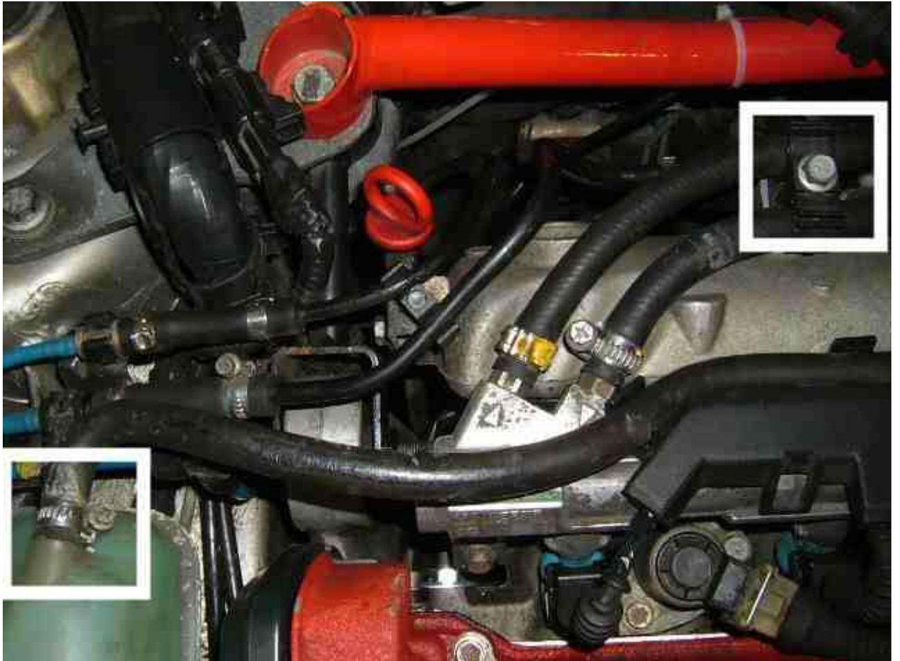
Remove the small hose attached to the fuel pressure regulator, shown here:
