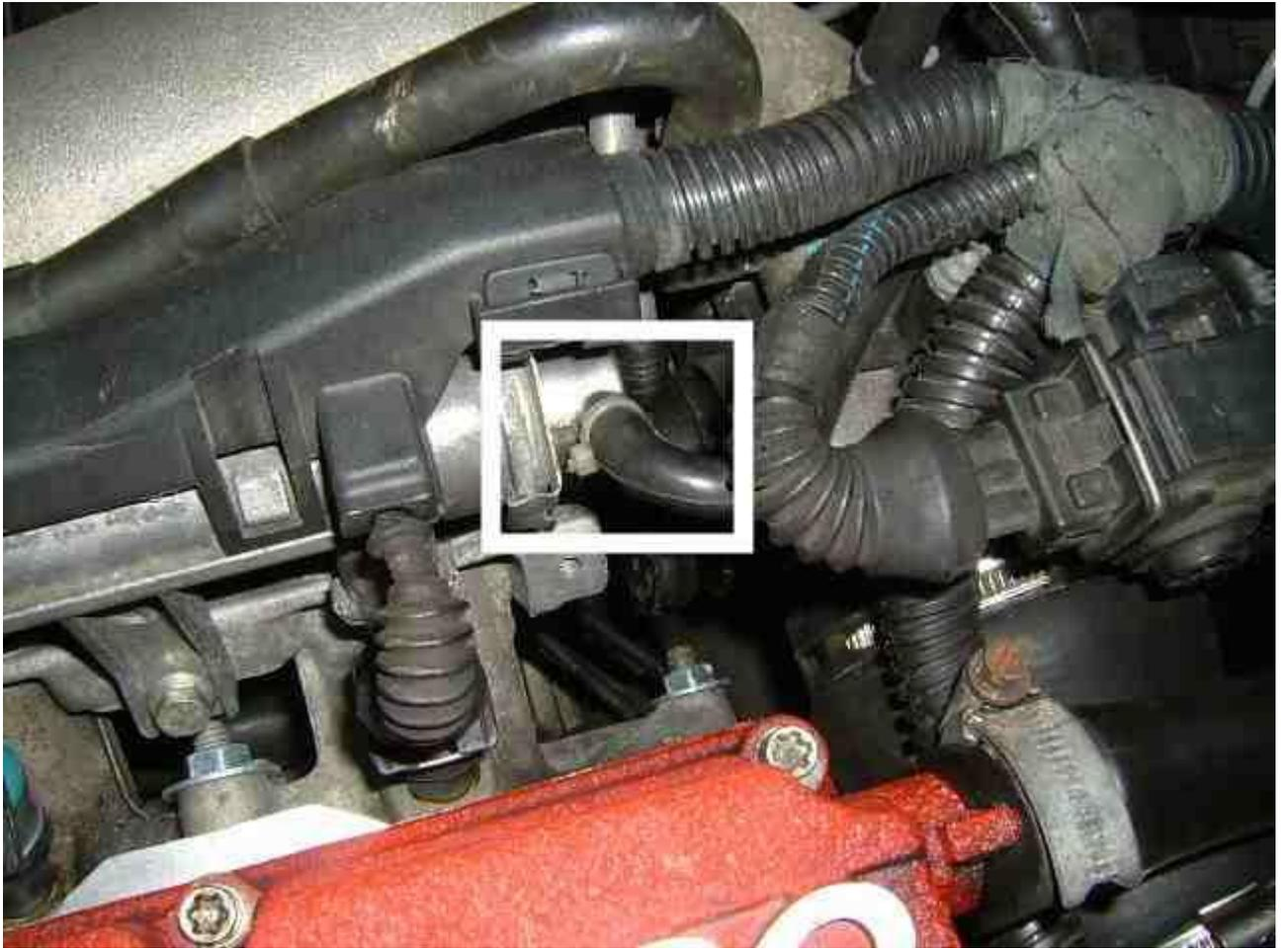
Release all the clips holding the plastic cover on top of the fuel rail which will allow you to move all the wires + the coolant hose out of the way (see picture below)
