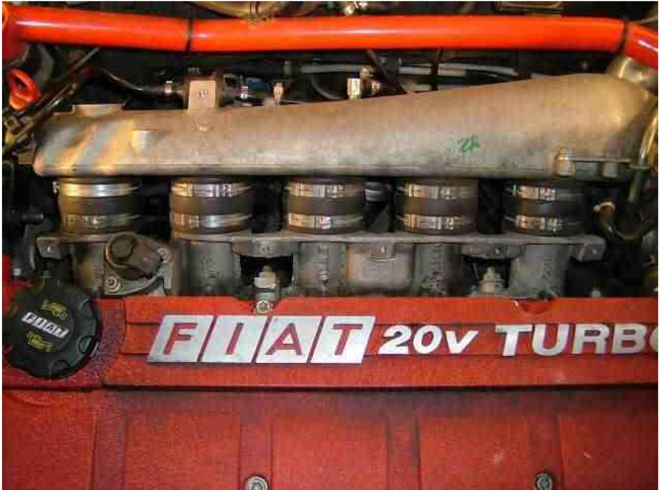
The next step will cause petrol to leak out of the rail, so get a big, thick rag and put it on top of the spark plug cover to soak up the spillage.
