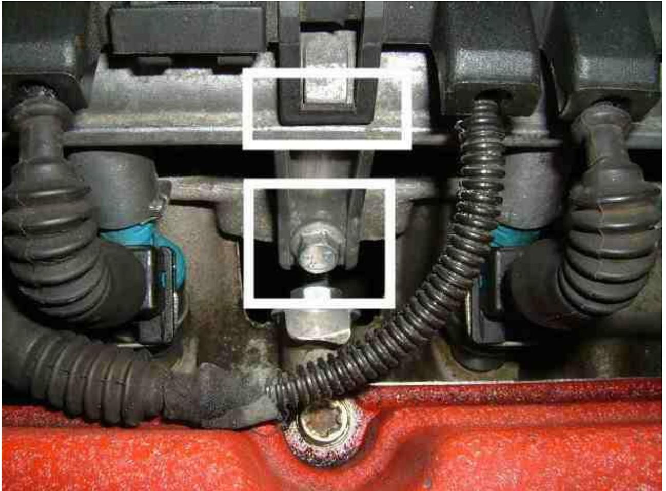
The entire fuel rail, complete with injectors, should now pull up/away from the intake manifold and be left attached only by the 2 fuel lines. The o-rings are very tight so it can need quite a strong pull.
