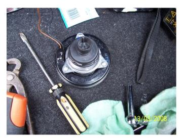
Just on the inner part of the cup there is a lip superglue this and push the lights into place, make sure that the Hella sign is straight up, and that's it the wiring is really easy,
