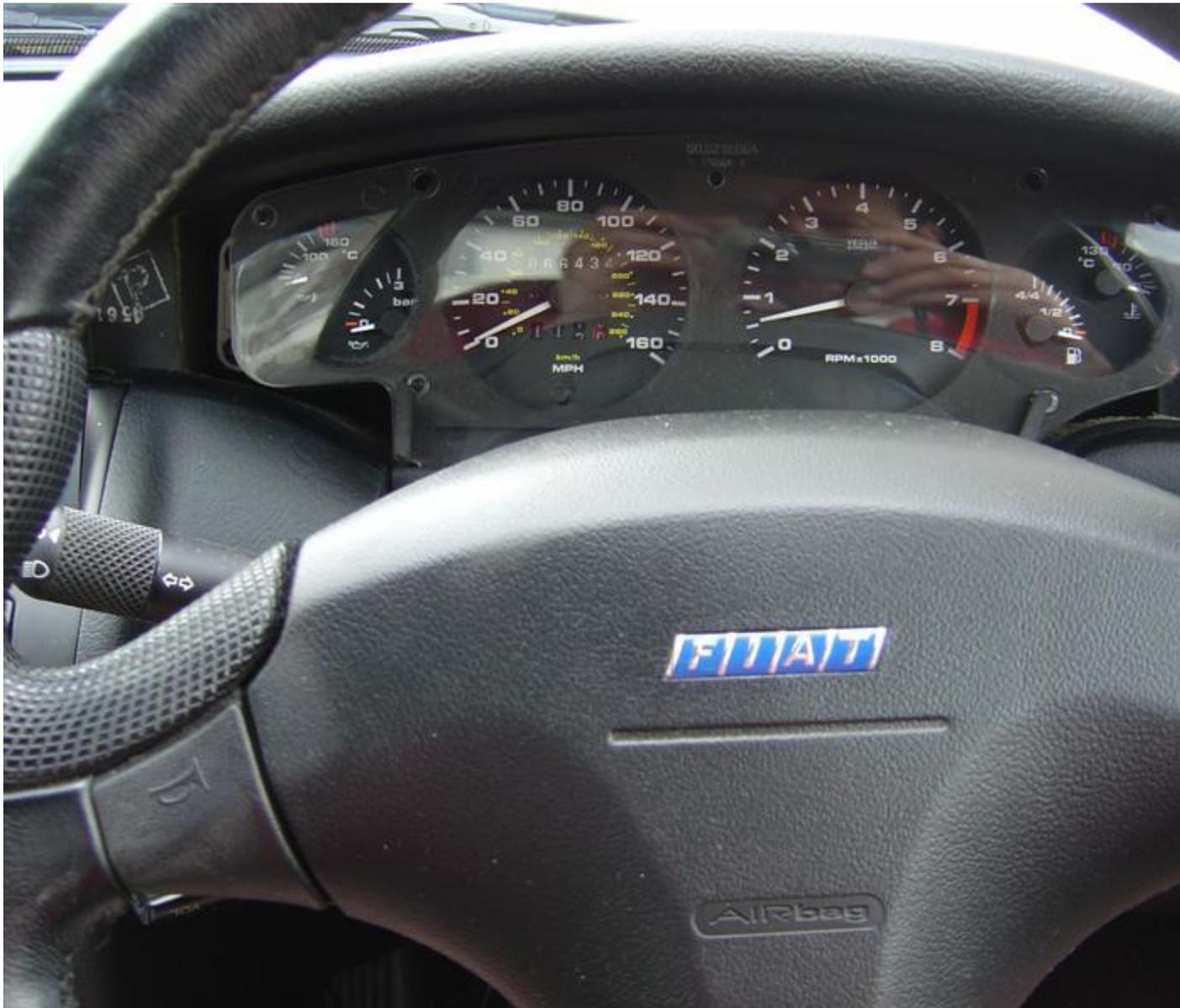
*BEFORE* undoing the 4 cross head screws mark the position of the instruments. Otherwise when you replace everything the warning lights and some of the gauges will not line up properly.
