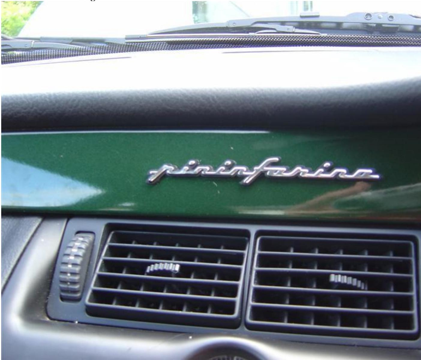
Here are some of the suggested ways of doing this. To understand why the badge is so difficult to remove it is handy to see how it is attached. The two clips are hard to remove and can dig into the pins of the badge, making removal an unnecessarily difficult procedure
