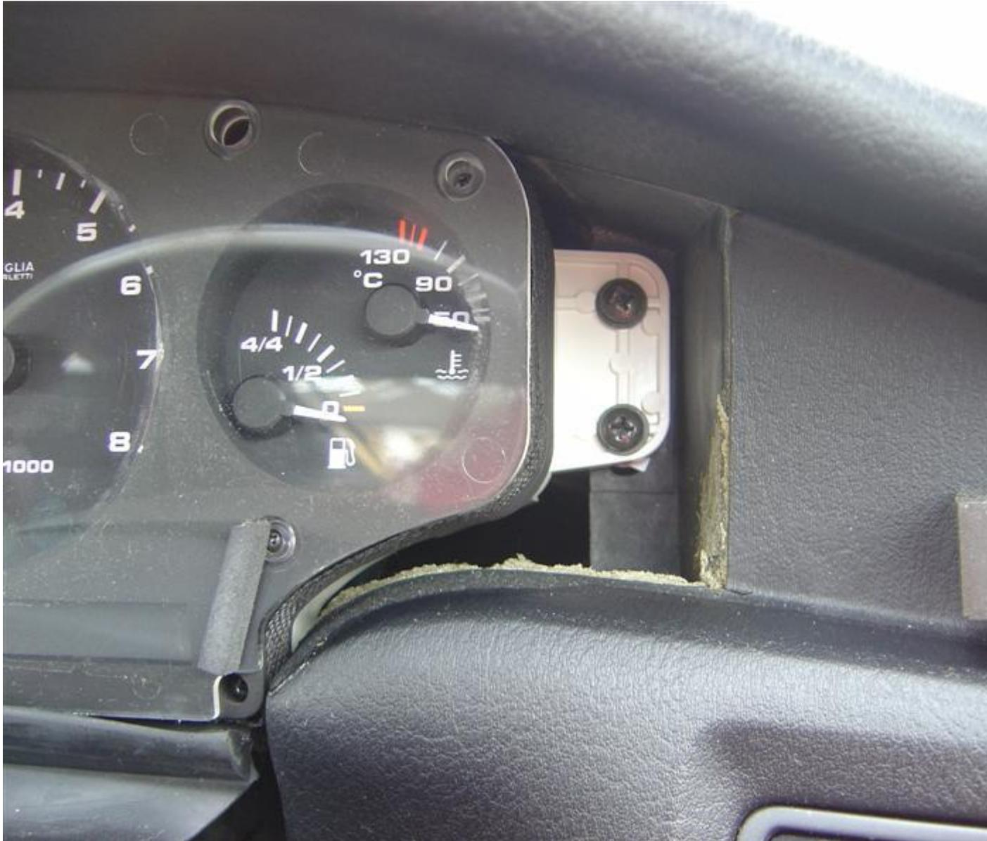
Once the 4 cross head bolts are removed the instrument panel can be pulled forward. This gives you just enough room to get your hands behind to release the catches, but these are a complete pain to get at and can be quite difficult to release. Don't worry too much about what plugs go where as they are all unique and only fit in one way.
