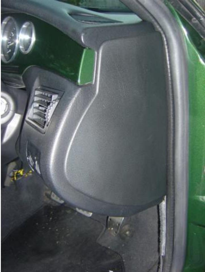
These are removed by undoing this knurled nut and removing the plastic clip
