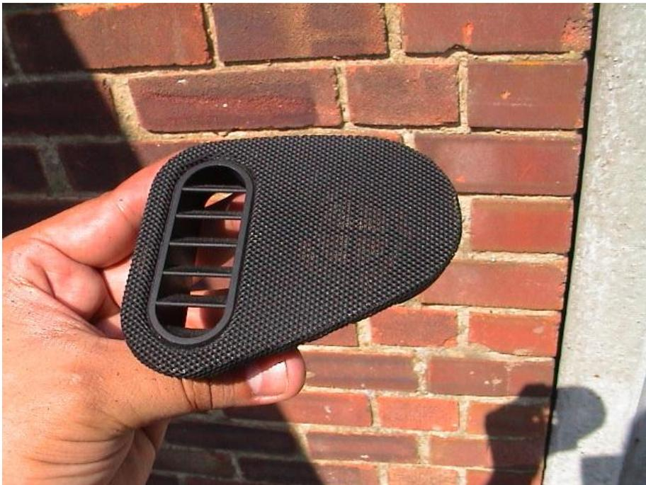
Remove the standard tweeter by twisting it anticlockwise off.
