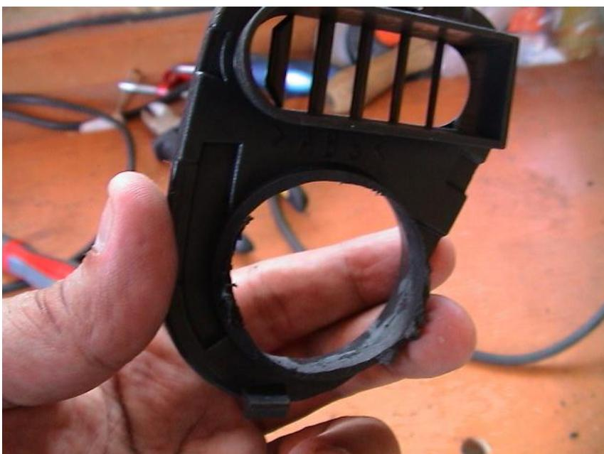
Not too much modification to do on the 0.75" tweeter then. The 1" tweeter needs a hole from nearly the edge of the housing to the air vent, and is very tricky to get it right.
